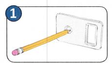
Do not remove the protective covering from the adhesive back at this time. Use the actual panel as a template to locate and mark the rotary timer switch and master switch mounting hole.
